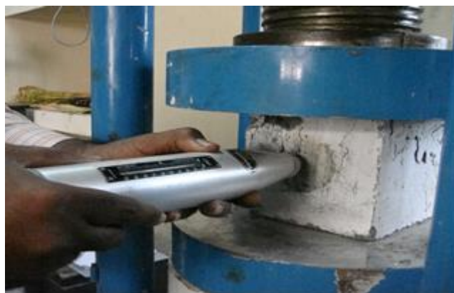
Figure 8 Rebound Hammer Test
