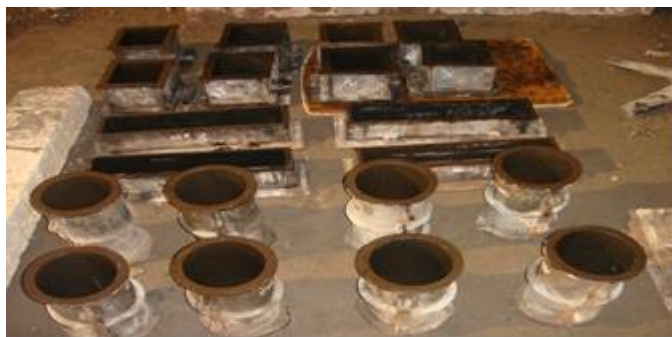
Figure 3 Moulds for Casting
