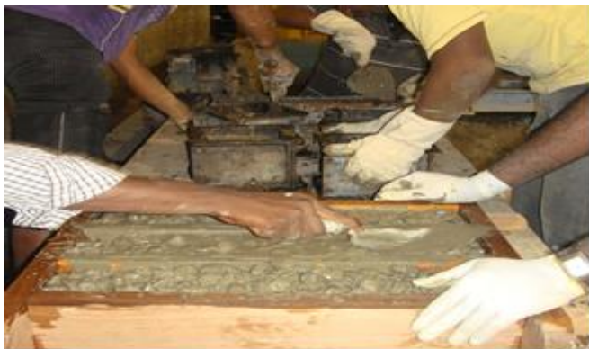
Figure 5 Placing of Concrete
